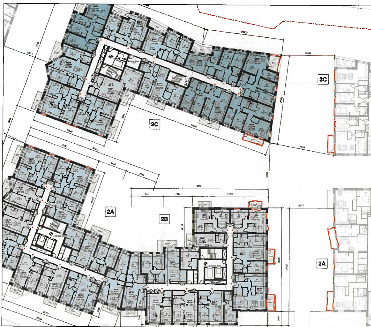
Figure 2: Extract of Block 2A,2B,2C (Zone 2) Plan at First Floor (Drawing No. DD-GRID-02-01-DR-A-PL121, Rev. P01) with windows and balconies (in red) where undue overlooking is deemed to potentially occur given separation distances of less than 20m.
