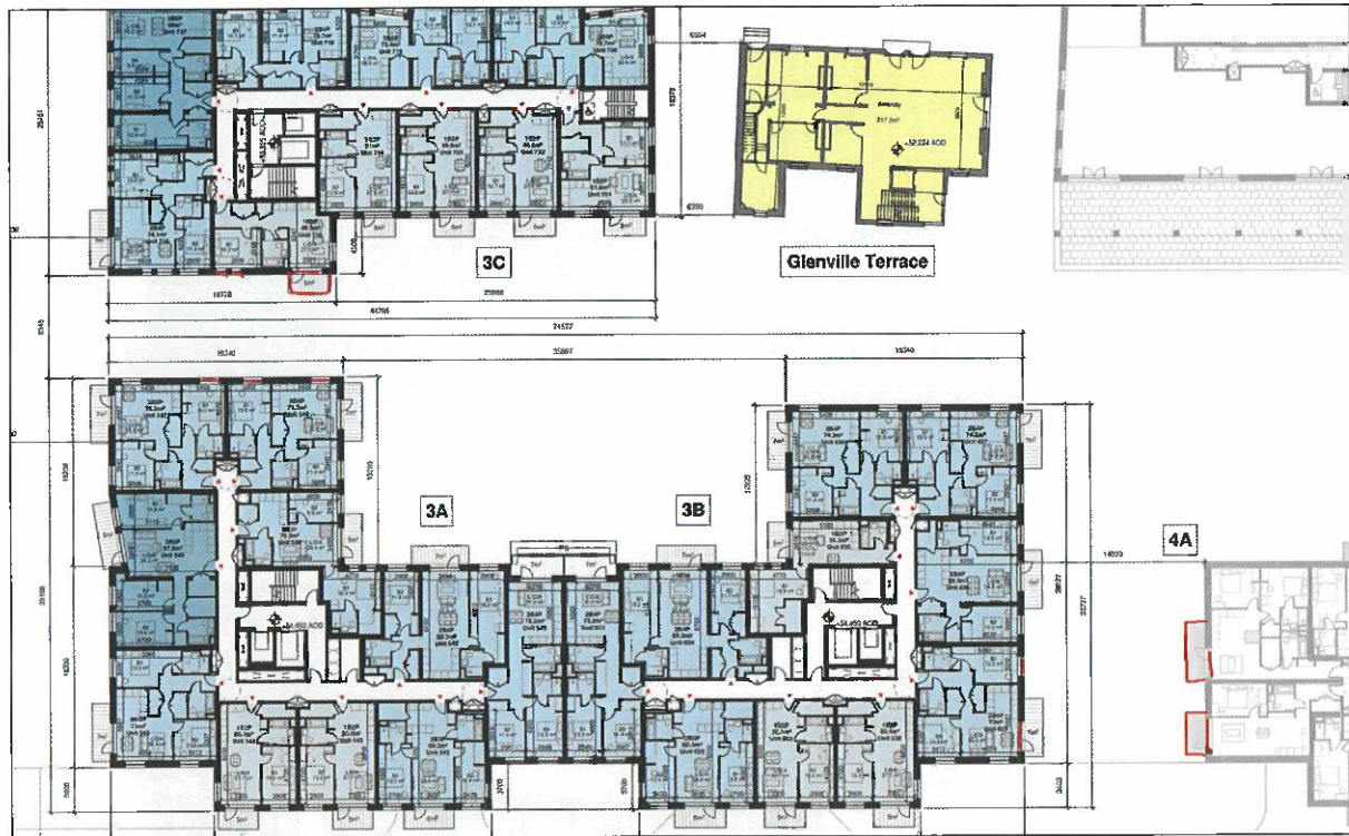
Figure 3: Extract of Block 3A,3B,3C (Zone 3) Plan at First Floor (Drawing No. DD-GRID-03-01-DR-A-PL141, Rev. P01) with windows and balconies (in red) where undue overlooking is deemed to potentially occur given separation distances of less than 20m.
